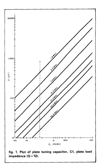
dances simply by linearly interpolating. For example, if the value of capacitor C1 is needed for a load impedance half way between 1500 and 2000 ohms on the 160 meter band, take the arithmetic mean:
